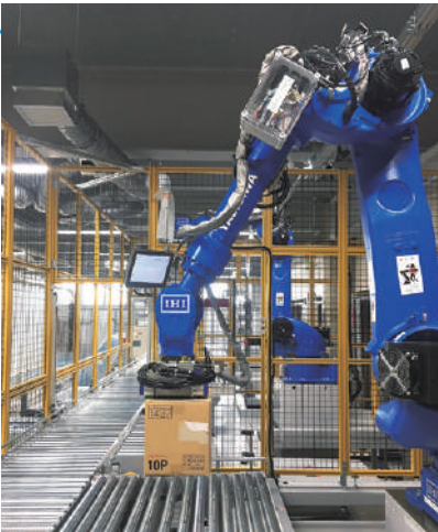
AI depalletizing robots: Two robots are capable of processing 900 cases per hour.
